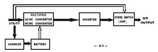
When Utility is normal, the AC source is rectified to DC, partially fed into the charger to charge battery and partially fed into inverter. The inverter reverts the DC to AC to supply energy to the load connected. The Utility LED and Inverter LED Light up.
