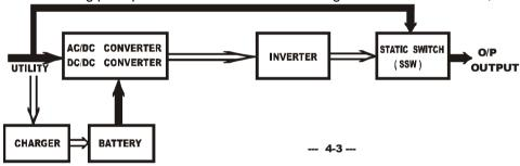
Normally, an inrush current is generated when switching on the connected device. If the UPS is in 105~120% loading, it will switch to bypass mode in 60 seconds. If The UPS is in 120%-150% loading, it will switch to bypass mode in 10 seconds. If The UPS is over 150% loading, it will switch to bypass mode immediately. The Utility LED, Bypass LED and Over Load LED light up. If overload condition is eliminated by reducing the load to 80%~90%, the UPS will switch back to Inverter mode automatically.
