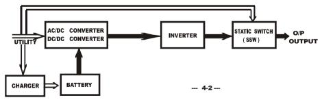
When Utility is abnormal, the UPS will use the battery energy automatically to energize the Inverter, and turn off the charger and AC/DC converter. The inverter revert DC to AC to supply energy to the output load connected. The Inverter LED lights up.
